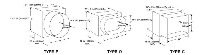
\* These dimensions are furnished approximately <sup>1</sup>/<sub>4</sub> in. (6mm) undersize, except round and oval dimensions which are approximately <sup>1</sup>/<sub>8</sub> in. (3mm) undersize.
